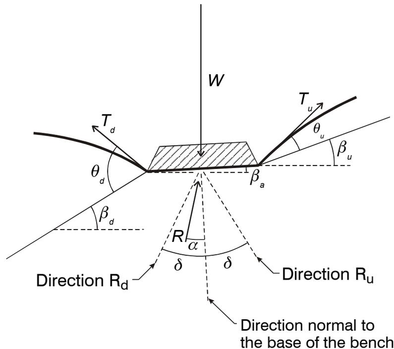
**Figure 5. Forces acting on an anchor bench when the geomembrane is uplifted by wind action.**
