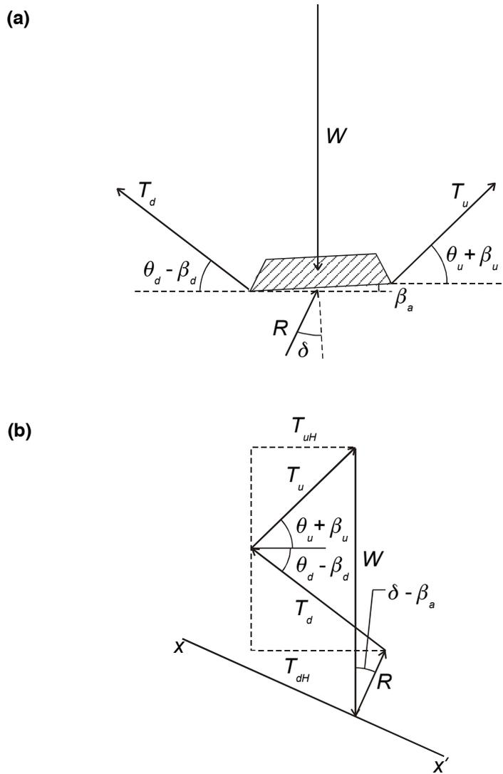
Figure 7. Case of anchor bench failure by sliding in the downslope direction: (a) forces acting on the anchor bench; (b) force diagram.
