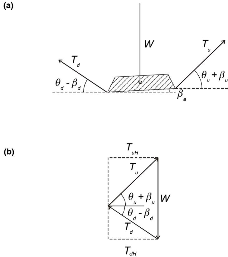
Figure 9. Case of anchor bench failure by uplifting: (a) forces acting on the anchor bench; (b) force diagram.
