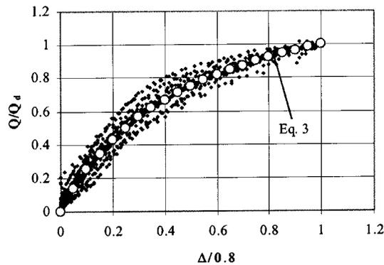
Fig. 9. Load-slip relation for shear studs
