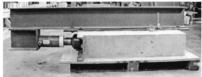
Fig. 4. Side view of pushout test setup
