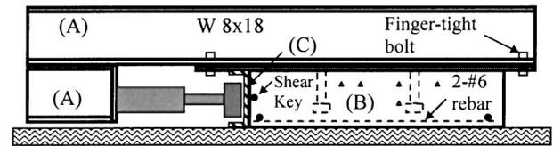
Fig. 3. Schematic of pushout test setup
