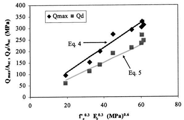
Fig. 16. Stud strength results and recommendations
