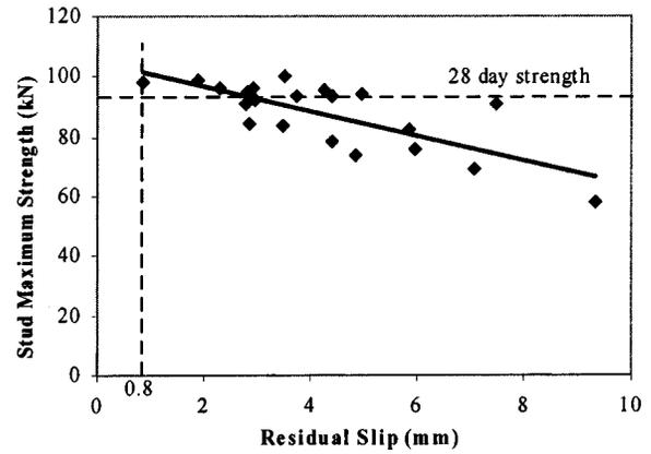
Fig. 13. Residual slip versus maximum strength for retested specimens
