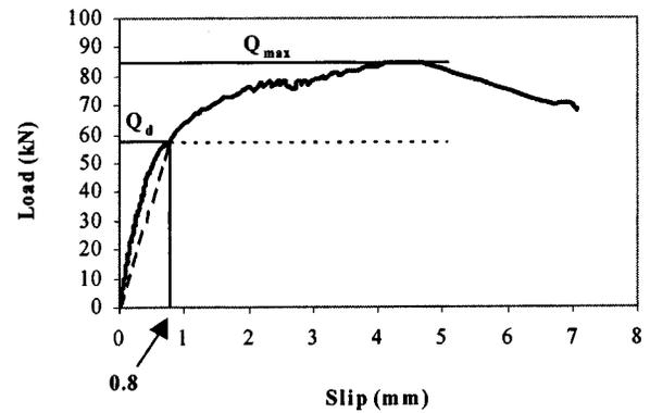
Fig. 8. Definition of design and maximum strength
