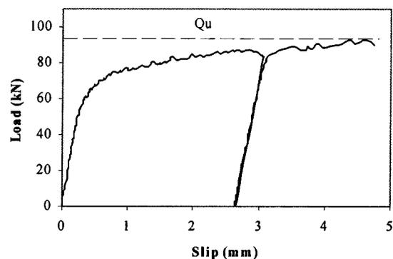
Fig. 2. Typical load-slip response for shear stud
