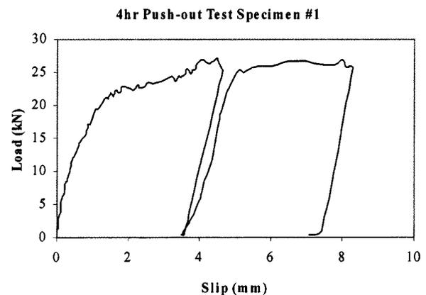
**Fig. 6.** Typical pushout test result
