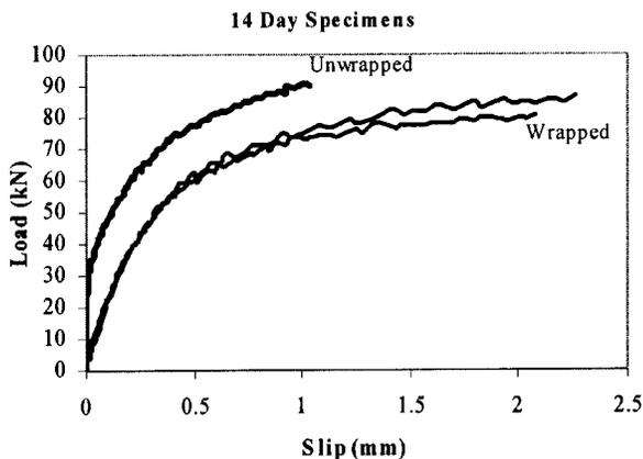
Fig. 15. Effect of steel surface treatment on stud behavior
