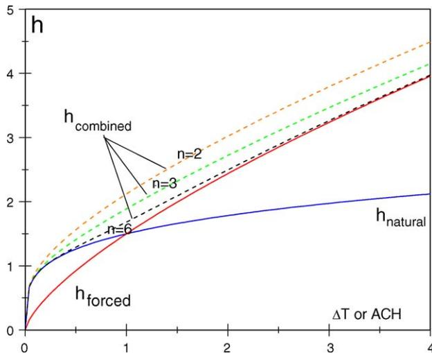
Fig. 3. Graphical interpretations for combined effects of forced and natural convection.
