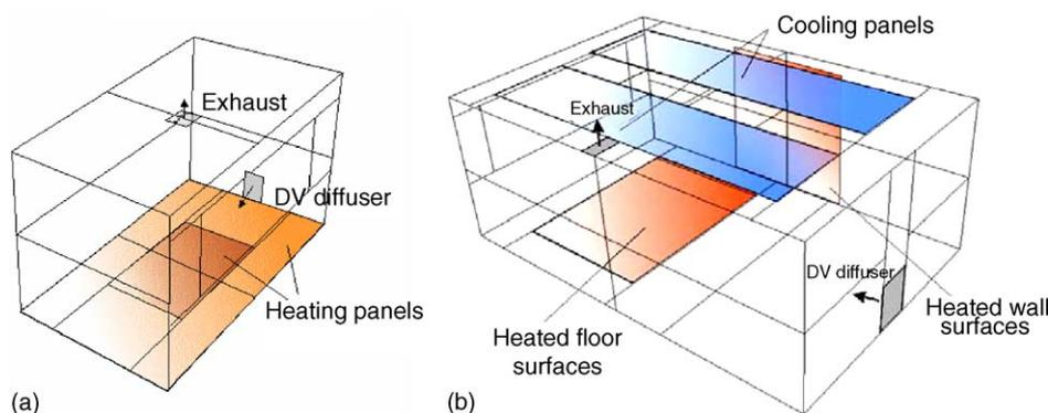
Fig. 4. Schematics of building environmental simulation and testing facility chambers: (a) climate chamber and (b) environmental chamber.
