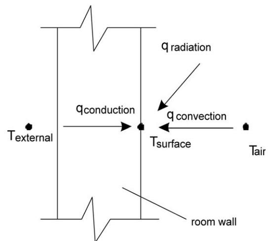
Fig. 2. The energy balance at an internal wall surface used to develop convection correlations.
