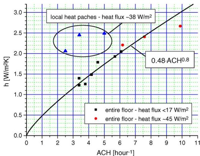
Fig. 9. Forced convection correlations for the floor with a DV diffuser including the convection coefficients measured at the heat patch floor area.
