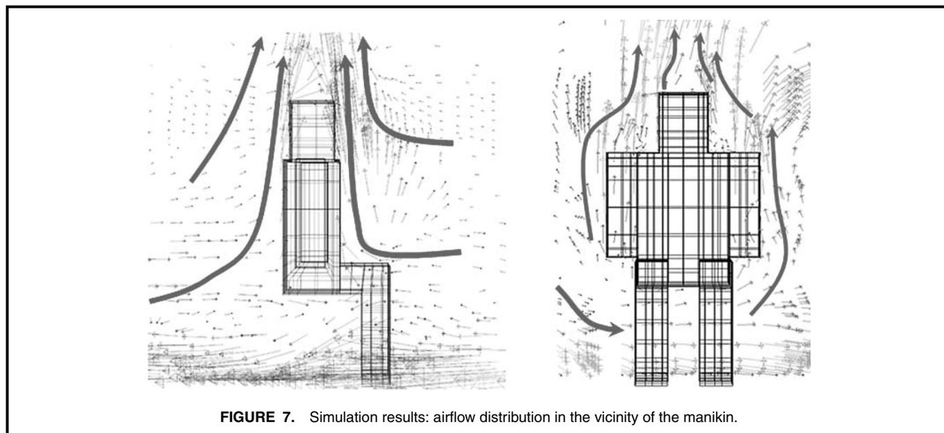
**FIGURE 7.** Simulation results: airflow distribution in the vicinity of the manikin.
