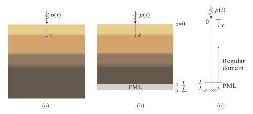
Figure 1. Prototype 1D problem (a) Original domain: horizontally-layered heterogeneous semi-infinite soil medium. (b) PML-truncated finite soil domain. (c) One-dimensional schematic of the PML-truncated domain (PML is placed at x = L and the PML's outer boundary is fixed at  $x = L_t$ ).
