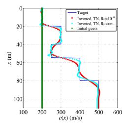
Figure 9. Inverted sharp 5-layer profile using Tikhonov regularization; fixed regularization factor versus regularization factor continuation scheme.
