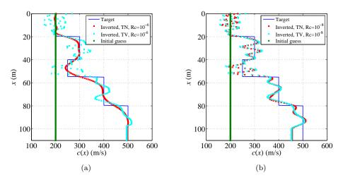
Figure 11. Inverted 5-layer profile using measured data with 20% Gaussian noise. Both TN and TV regularization schemes were used with: (a)  $R_c = 10^{-6}$ , and (b)  $R_c = 10^{-8}$ .
