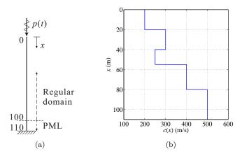
Figure 6. A target wave velocity profile with 5 layers.
