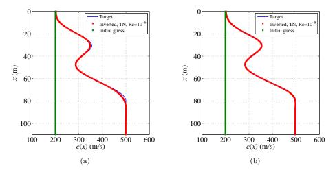
Figure 4. Initial guess, target, and inverted wave velocity profiles using Tikhonov regularization with: (a)  $R_c = 10^{-6}$ , and (b)  $R_c = 10^{-8}$ ; both results were obtained using 3760 iterations.
