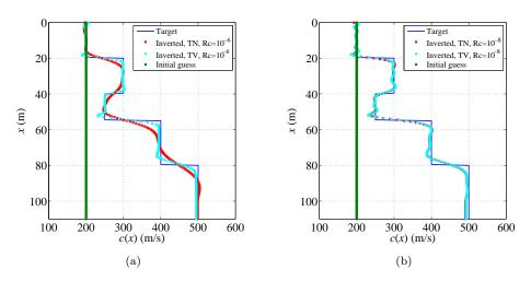
Figure 8. Inverted sharp 5-layer profile using Tikhonov and Total Variation regularization with: (a)  $R_c = 10^{-6}$ , and (b)  $R_c = 10^{-8}$ ; both results were obtained using 2660 iterations.
