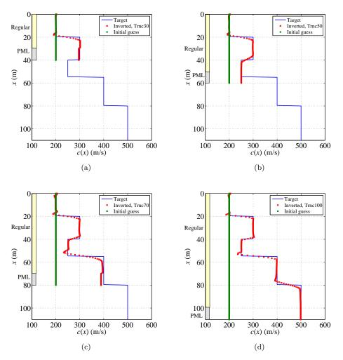
Figure 12. Target, initial guess, and estimated wave velocity profiles c(x) with PML location at (a) 30m; (b) 50m; (c) 70m; (d) 100m; observation period T is optimized; measured data are noise-free.
