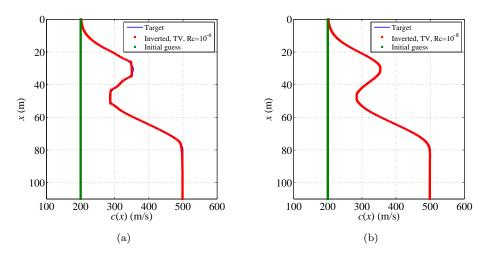
Figure 5. Initial guess, target, and inverted wave velocity profiles using Total Variation regularization with: (a)  $R_c = 10^{-6}$ , and (b)  $R_c = 10^{-8}$ ; both results were obtained using 5000 iterations.
