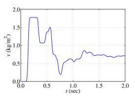
Figure 7. Measured displacement response v(0, t). Data are obtained by applying the stress load p(t) presented in figure 3(a) on the 5-layer profile depicted in figure 6(b).
