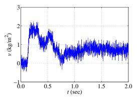
Figure 10. Measured displacement response v(0,t) with 20% Gaussian noise. Data are obtained by applying the stress load p(t) presented in figure 3(a) on the 5-layer profile depicted in figure 6(b).
