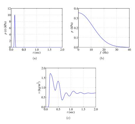
Figure 3. (a) Time history of the applied stress p(t). (b) Frequency spectrum of the applied stress p(t). (c) Measured displacement response  $v(0,t) (= \rho u(0,t))$ .
