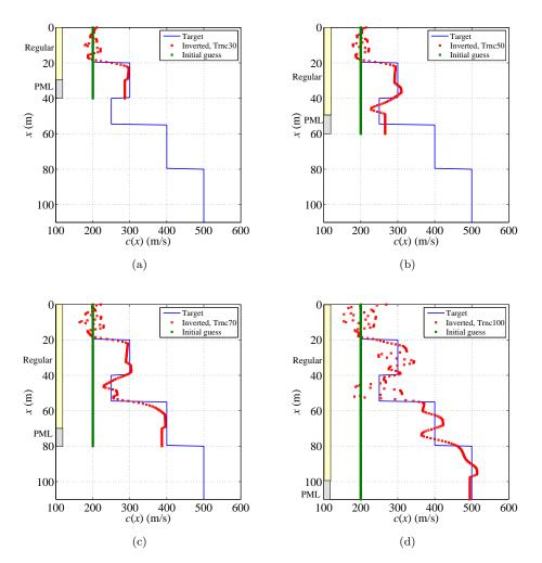
Figure 13. Target, initial guess, and estimated wave velocity profiles c(x) with PML location at (a) 30m; (b) 50m; (c) 70m; (d) 100m; observation period T is optimized; measured data with 20% Gaussian noise.
