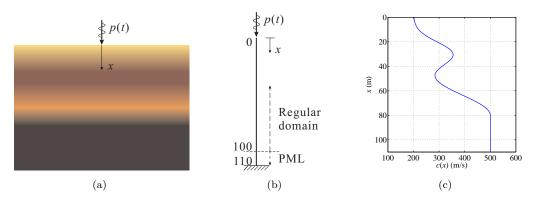
Figure 2. (a) Heterogeneous semi-infinite soil medium; (b) corresponding one-dimensional PML-truncated semi-infinite domain; (c) target, smooth, wave velocity profile c(x)
