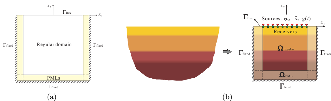
Figure 1. (a) A PML-truncated semi-infinite domain in two dimensions; (b) conceptual configuration of material profile reconstruction in a PML-truncated semi-infinite domain
