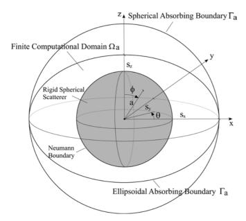
Fig. 4 Model of rigid scatterer surrounded by an absorbing boundary
