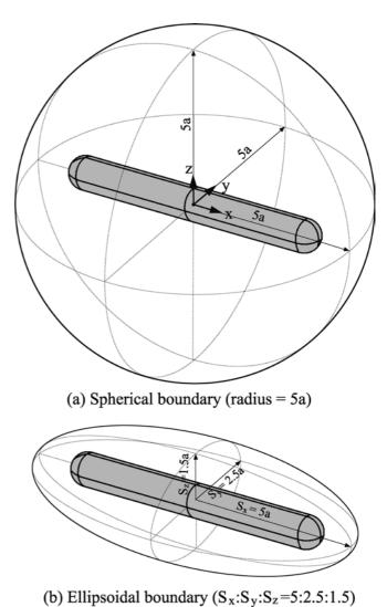
Fig. 6a, b Geometry of absorbing boundaries for finite cylinder problem
