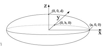
Fig. 2 Ellipsoidal absorbing boundary geometry
