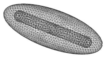
Fig. 3 Typical tetrahedral mesh over the bounded computational domain  $\Omega_a$ ; shown are the element traces on the absorbing boundary and the scatterer surface
