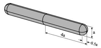
**Fig. 5** Geometry of elongated scatterer; dimensional ratio along the median axes is 8:1:1
