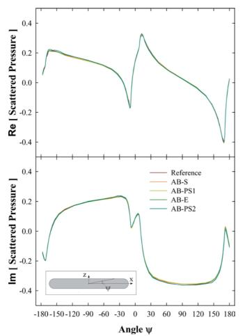
Fig. 8 Real and imaginary parts of scattered pressure on the surface of the scatterer along the *xz*-plane due to oblique incidence ( $P_{i_{125}}$ )
