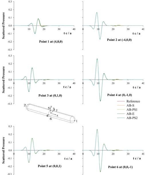
ka = 1 is  $2\pi a$ . That is, the boundary is, approximately, 0.08 wavelengths away from the scatterer. Whereas, such a close placement may be too tight for applications, we believe that, based on numerical experiments not reported herein, satisfactory results can be obtained with boundaries placed at 0.2 of the dominant wavelength (still at only a fraction of a wavelength).
