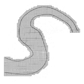
FIG. 1. Channel Bend with Square Cartesian Mesh
