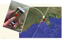
Pin2Flood is currently two apps—one for field responders (pins drops, flood extent) and one for emergency managers (pins, flood extent, export). With both apps simultaneously displaying the same data, the result is a common operating picture with real-time flood impact maps.
