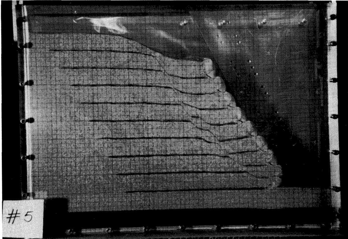
*Failure of a geotextile-reinforced slope model, as obtained after testing in a geotechnical centrifuge.*
