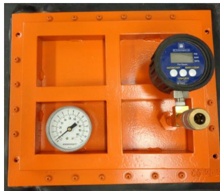
Figure 2.5 Refined normal pressure control system
