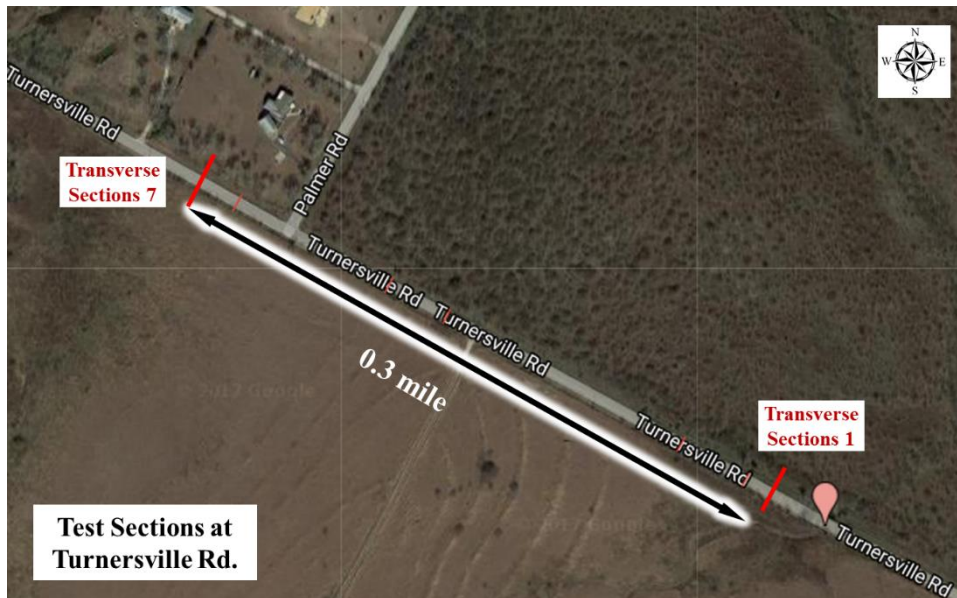
Figure 4.50 Layout of test sections at Turnersville Road
