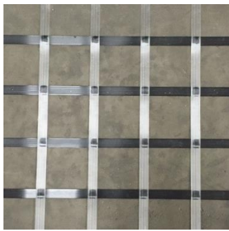
Figure 3.4 Baseline biaxial laser-bonded geogrid from polypropylene: GG 4
