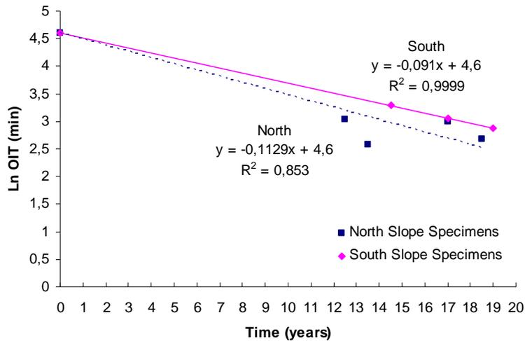
Figure 6. Ln(OIT) versus ageing time for Std-OIT Test.
