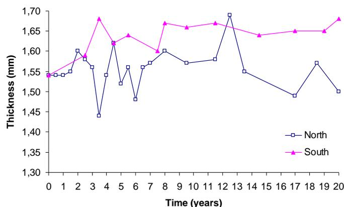
Figure 2. Evolution of the thickness in north and south samples extracted in the crest area.
