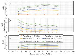
Figure 3. Reinforcement nodal displacement: (a) Main layer; (b) Upper boundary layer; and (c) Bottom boundary layer
