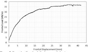
Figure 2. Frontal pullout load-displacement behavior
