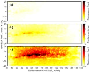
Figure 4. Horizontal displacement field: (a) at 7.4-kN/m frontal load; (b) at 19.1-kN/m frontal load; (c) at 35.9-kN/m frontal load Figure 5. Vertical displacement field: (a) at 7.4-kN/m frontal load; (b) at 19.1-kN/m frontal load; (c) at 35.9-kN/m frontal load
