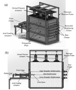
Figure 1. General layout of the new equipment: (a) 3D perspective; (b) sectional side view.
