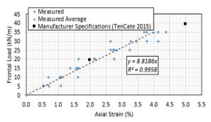
Figure 7. Reinforcement unconfined tensile behavior
