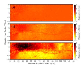
Six artificial gravel particles were stacked in a vertical array, centered in the box and located 30.5 cm (X = +30.5 cm) from the front wall to measure the horizontal deformation. Soil
