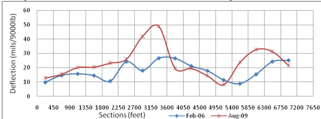
Figure 2. Comparison of average D<sub>0</sub> for the first and latest FWD testing surveys
