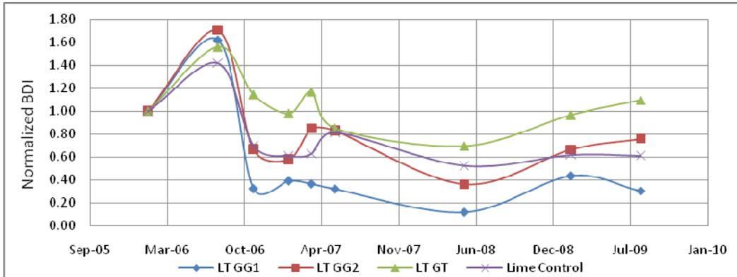
Figure 6. Variation of Normalized BDI for sections with only reinforcement
