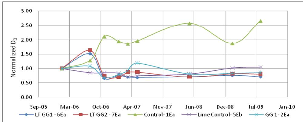
Figure 4. Variation of Normalized D<sub>0</sub> for various sections for 9 FWD field tests
