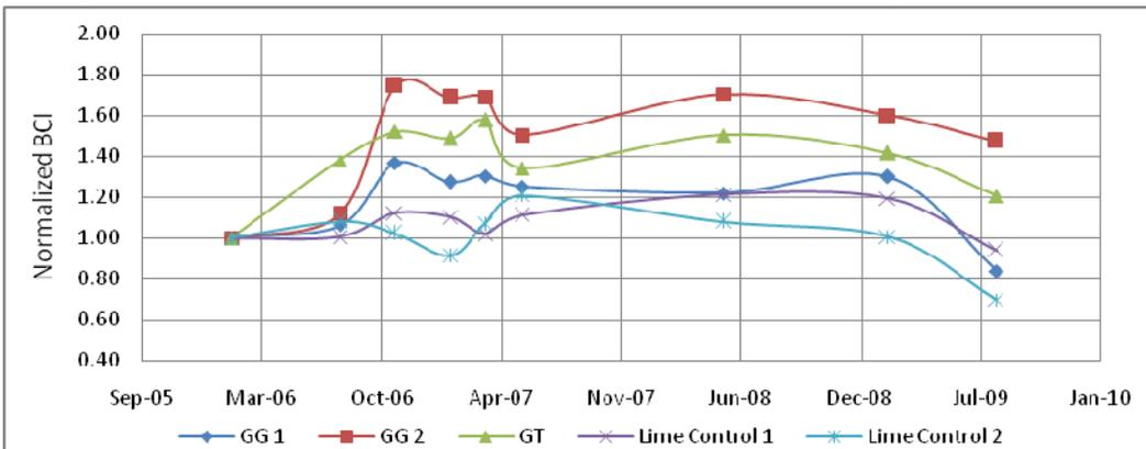
Figure 7. Variation of Normalized BCI for reinforced sections against lime control
