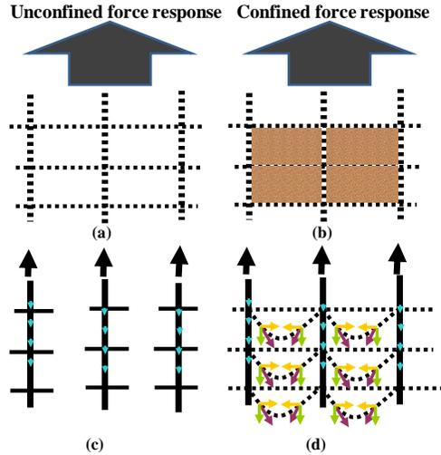
Figure 4. Response of geosynthetic: (a) Unconfined force (b) Confined force (c) Longitudinal ribs mobilized under unconfined loads (d) Both longitudinal and transverse ribs mobilized under confined loading conditions
