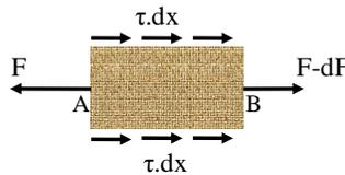
Figure 3. Free body diagram for geosynthetic element of length  $dx$  in pullout test
