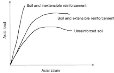
Figure 2. Axial load-strain relationship for various reinforcements with soil (McGown et al., 1978)
