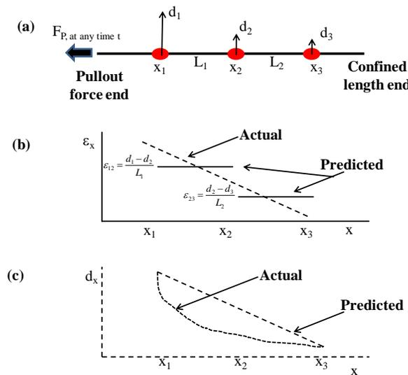
Figure 5. Predictions based on constant strain distribution: (a) Schematic of displacement profile for given pullout force (b) actual vs. predicted strain distribution (c) actual vs. predicted displacement
