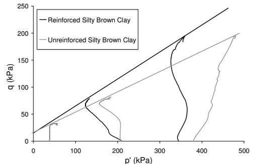
Figure 6: Stress Paths for Fiber-Reinforced and Unreinforced Silty Brown Clays Specimens from ICU Triaxial Testing.
