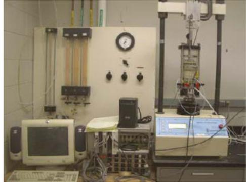
Figure 1: Photograph of the Triaxial Testing Setup.
