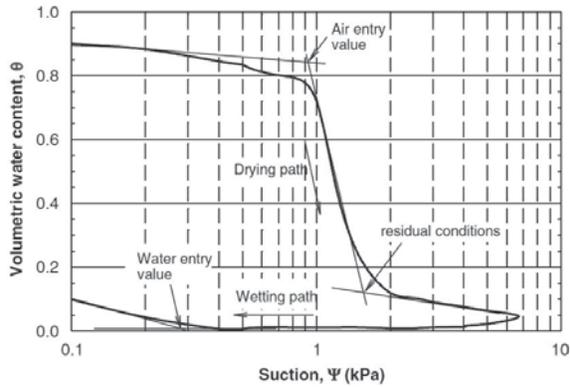
Figure 2. Typical geotextile WRC (Bouazza et al., 2006).
