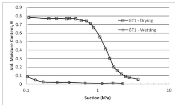
Figure 7. Water retention curve for GT1.
