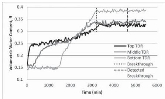
Figure 9. Example water content data from TDRs.
