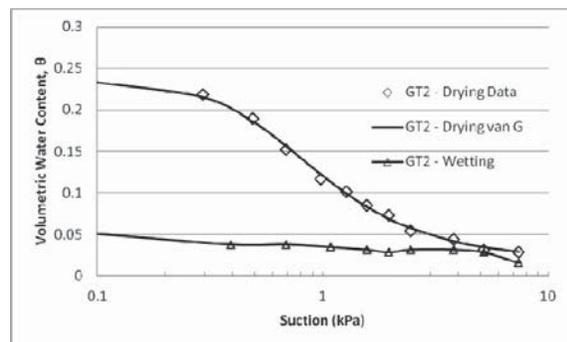
Figure 5. Water retention curve for GT2.
