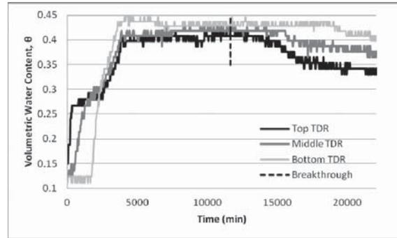
Figure 10. Dissipation of capillary barrier by GT5.
