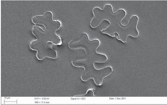
Figure 1. Typical 4DG wicking fiber cross-section.
