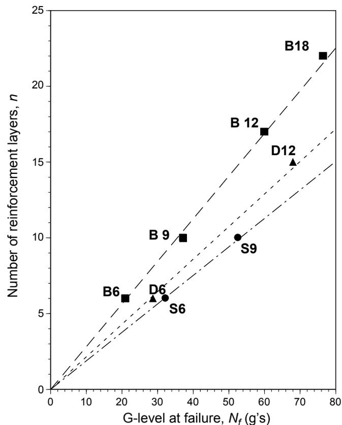
Figure 8. G-level at failure for the centrifuge models.
