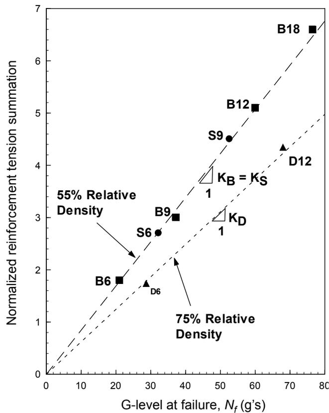
Figure 9. Normalized reinforcement tension summation values from centrifuge test results.
