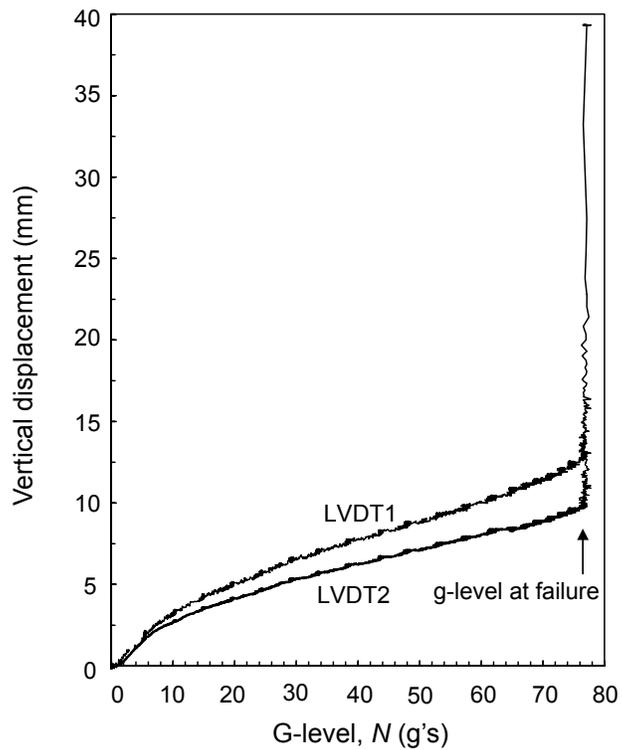
Figure 5. Settlements at the crest of a reinforced slope model.
