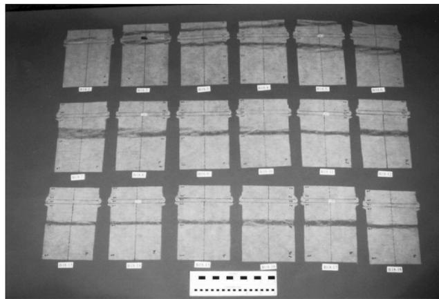
Figure 7. Geotextile reinforcements retrieved after testing.
