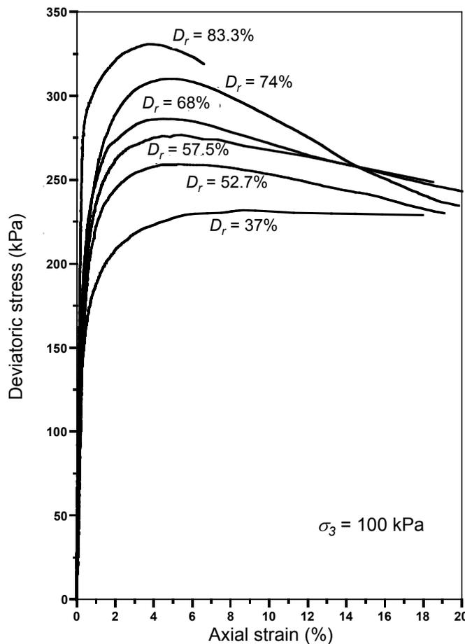
Figure 2. Stress strain behavior of Monterey No. 30 sand pluviated at different relative densities ( $D_r$ ) and tested in triaxial compression under the same confinement.
