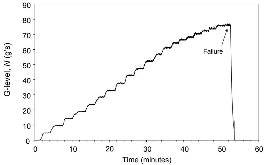
Figure 4. G-level,  $N$ , versus time during centrifuge testing.
