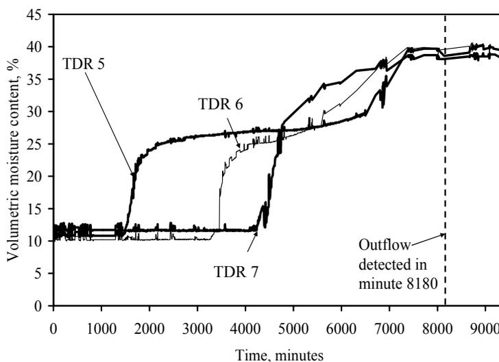
Figure 9: Volumetric moisture content with depth in Column 2.
