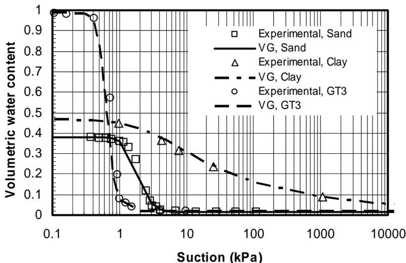
Figure 5: Soil and geocomposite hydraulic characteristics: Water retention curves (VG=van Genuchten equation).
