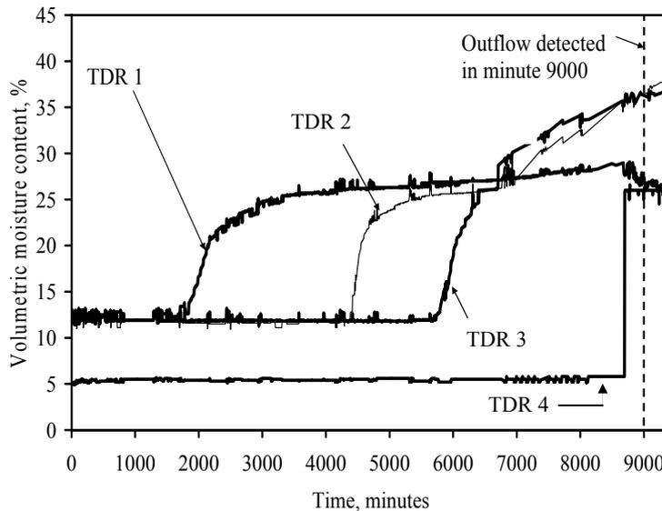
Figure 8: Volumetric moisture content with depth in Column 1.
