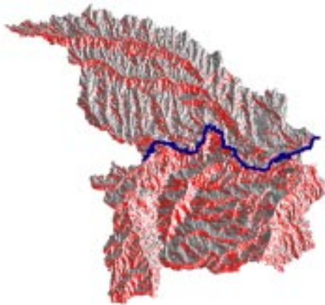
Figure 2.6 The flow direction grid for segment 841 with the corresponding segment grid on top
