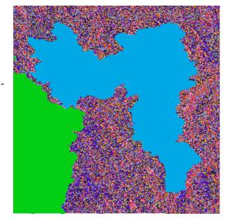
an input the Drainage Direction and as an output the Drin Basin, gives us the clipped Drainage Direction DEM with the Drin Basin
