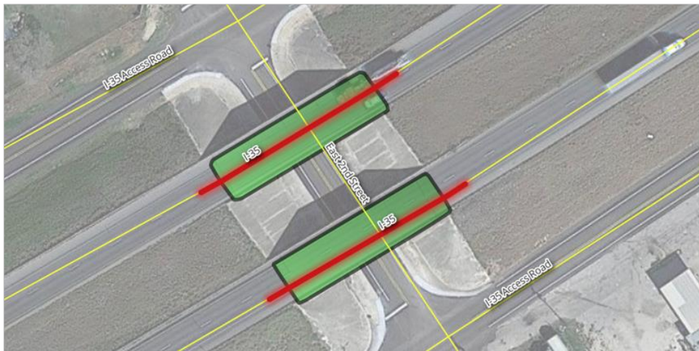
Figure 2.10 ‘Major Axis’ determined for bridge hulls using OpenStreetMap transportation linework
