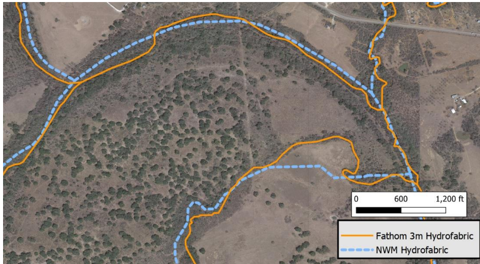
Figure 2.13 Comparison on the National Water Model and Fathom 3m Hydrofabric (N 28.971°, W 98.451°)
