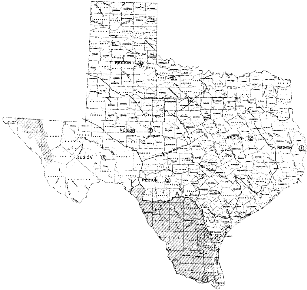
Figure 3-11 Hydrologic regions in Texas for regional regression equations Shaded areas are undefined. Adapted from TxDOT (1985, pp. 2-12)
