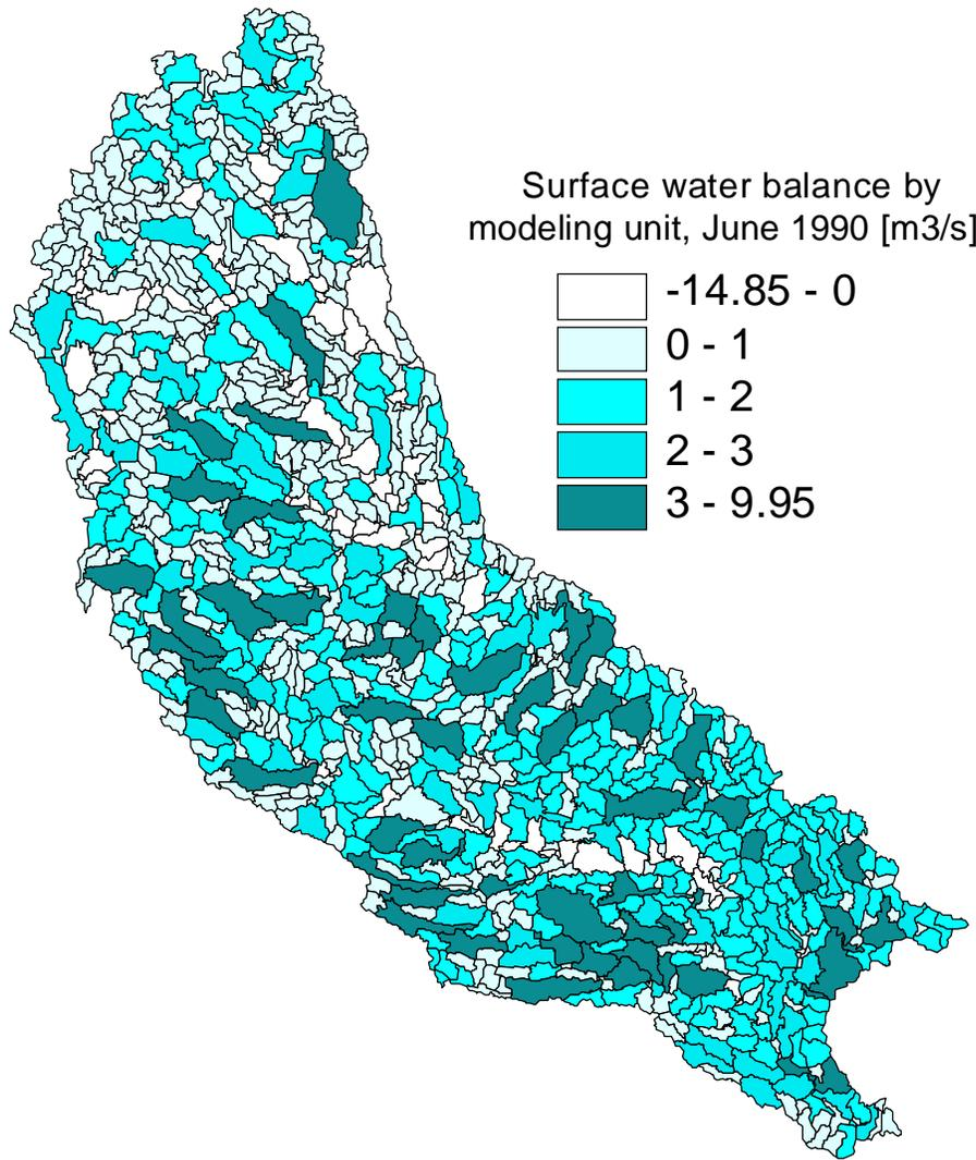
**Figure 6.12** Spatial distribution of the surface water balance for the modeling units. Estimated from recorded flow rate, precipitation depth and selected unit features, the Iowa-Cedar River basin, June 1990.
