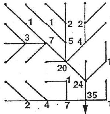
Figure 2.4: Creating a Drainage Network
