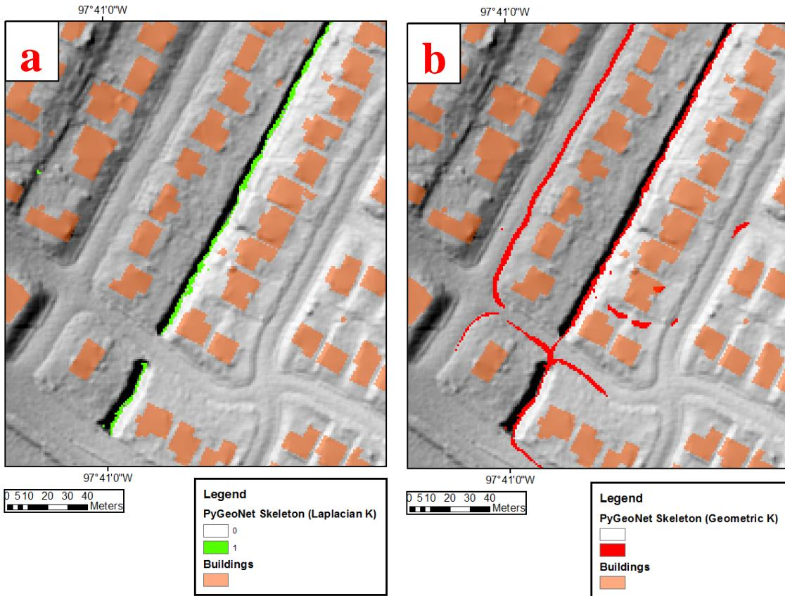
Figure 15. Python-based GeoNet channel skeletons for the 0.3 m resolution data using the Laplacian (a) and geometric (b) curvature computation methods. Note in b there are some locations where the channel network crosses through the buildings.
