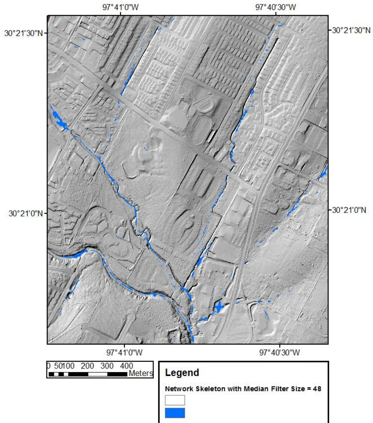
Figure 9. Channel skeleton results for median filter kernel size of 48 m (~3\* road width).
