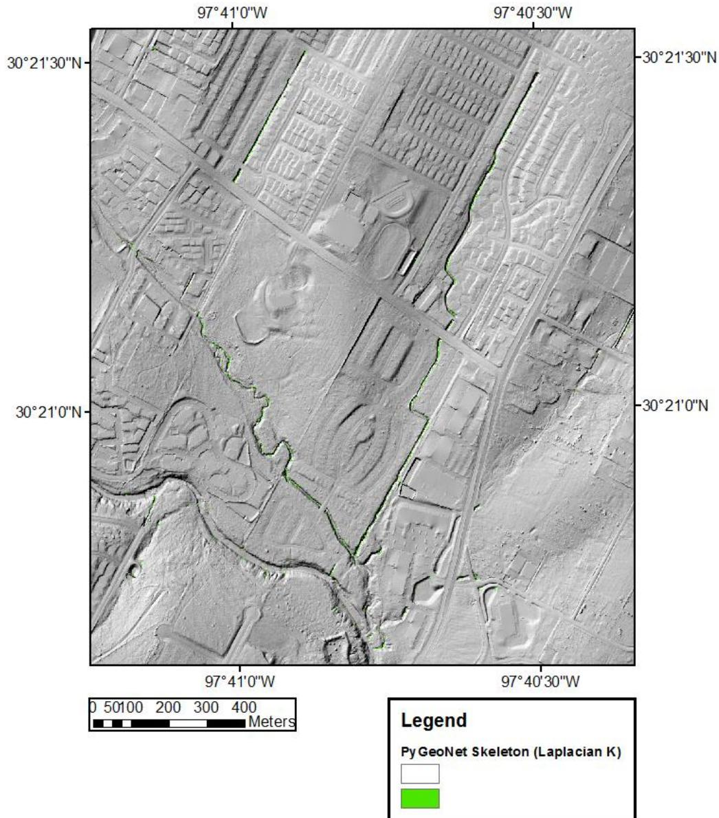
Figure 10. Python-based channel skeleton results for Laplacian curvature computation method.
