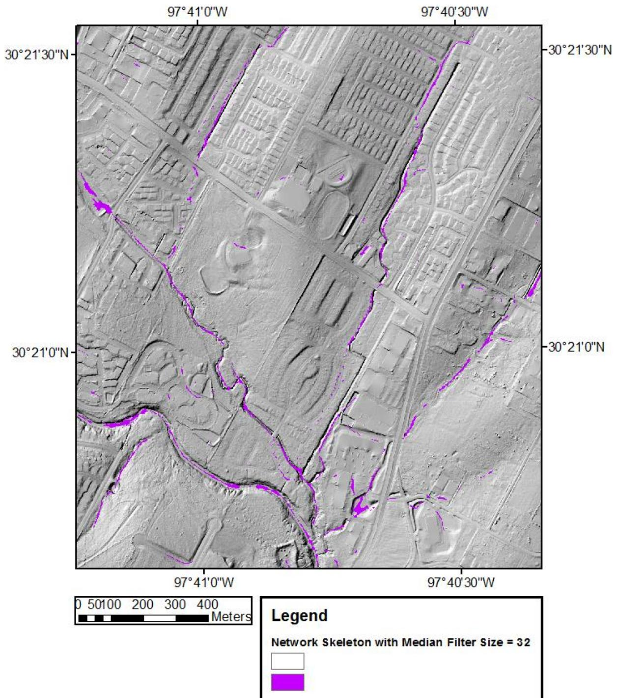
Figure 8. Channel skeleton results for median filter kernel size of 32 m (~2\* road width).
