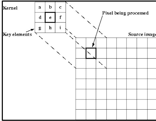
Figure 4. The median filter works via a kernel passing across the landscape and setting the centroid pixel, *e* in this example to the median of the values *a-i* within the kernel. Image source: [http://www2.hs-fulda.de/caelabor/inhalte/java/j3d/j3d\\_seminar/19/JAI%20Guide%20von%20Sun/Image-enhance.doc.anc5.gif](http://www2.hs-fulda.de/caelabor/inhalte/java/j3d/j3d_seminar/19/JAI%20Guide%20von%20Sun/Image-enhance.doc.anc5.gif)
