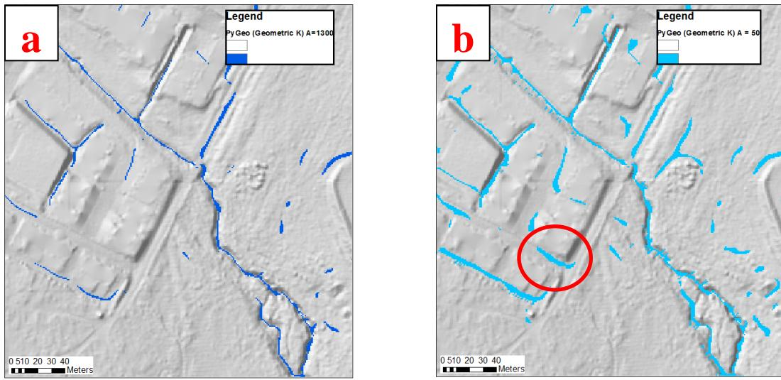
Figure 19. Python-based GeoNet channel skeletons for the 1 m resolution data using the geometric curvature. In (a) the results with the original flow accumulation area threshold of  $1300 \text{ m}^2$  are shown, in (b) the results with a threshold of  $50 \text{ m}^2$  is shown. The red circle highlights the flow contribution from the street in the residential area that is partially visible in the photo in Figure 17.
