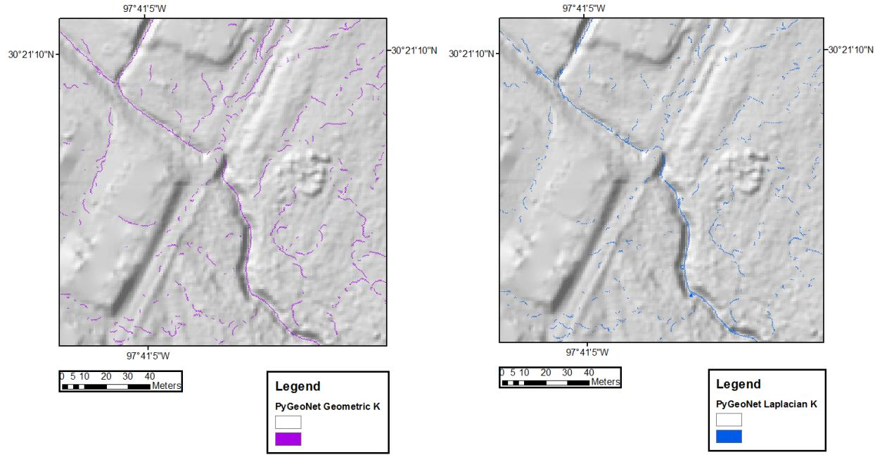
Figure 14. Channel skeleton results for 0.3 m resolution data for both curvature computation methods. This is a detailed view centered at the culvert that crosses Walnut Creek.
