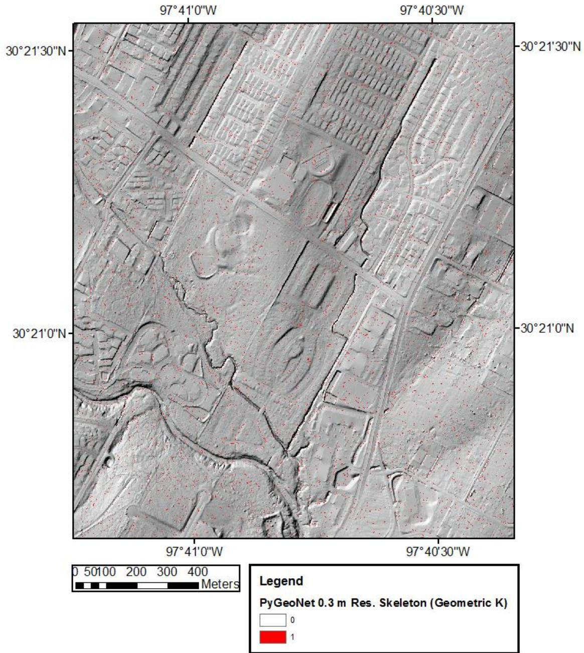
Figure 13. Python-based channel skeleton results for geomtric curvature computation method with 0.3 m resolution DEM.
