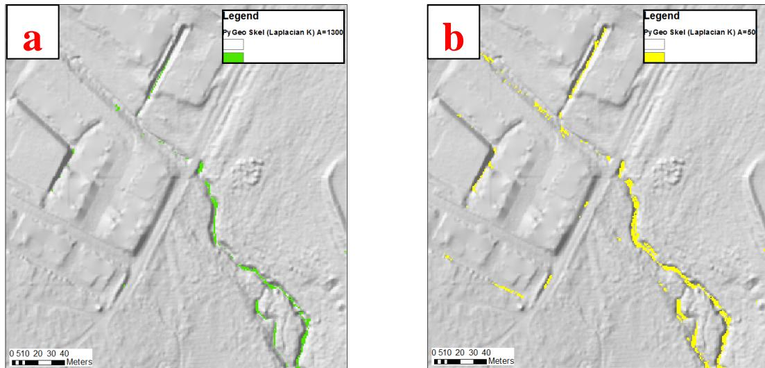
Figure 18. Python-based GeoNet channel skeletons for the 1 m resolution data using the Laplacian curvature. In (a) the results with the original flow accumulation area threshold of  $1300 \text{ m}^2$  are shown, in (b) the results with a threshold of  $50 \text{ m}^2$  is shown.
