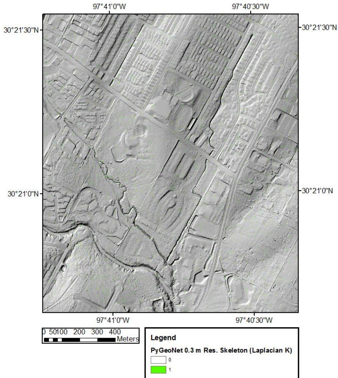
Figure 12. Python-based channel skeleton results for Laplacian curvature computation method with 0.3 m resolution DEM.
