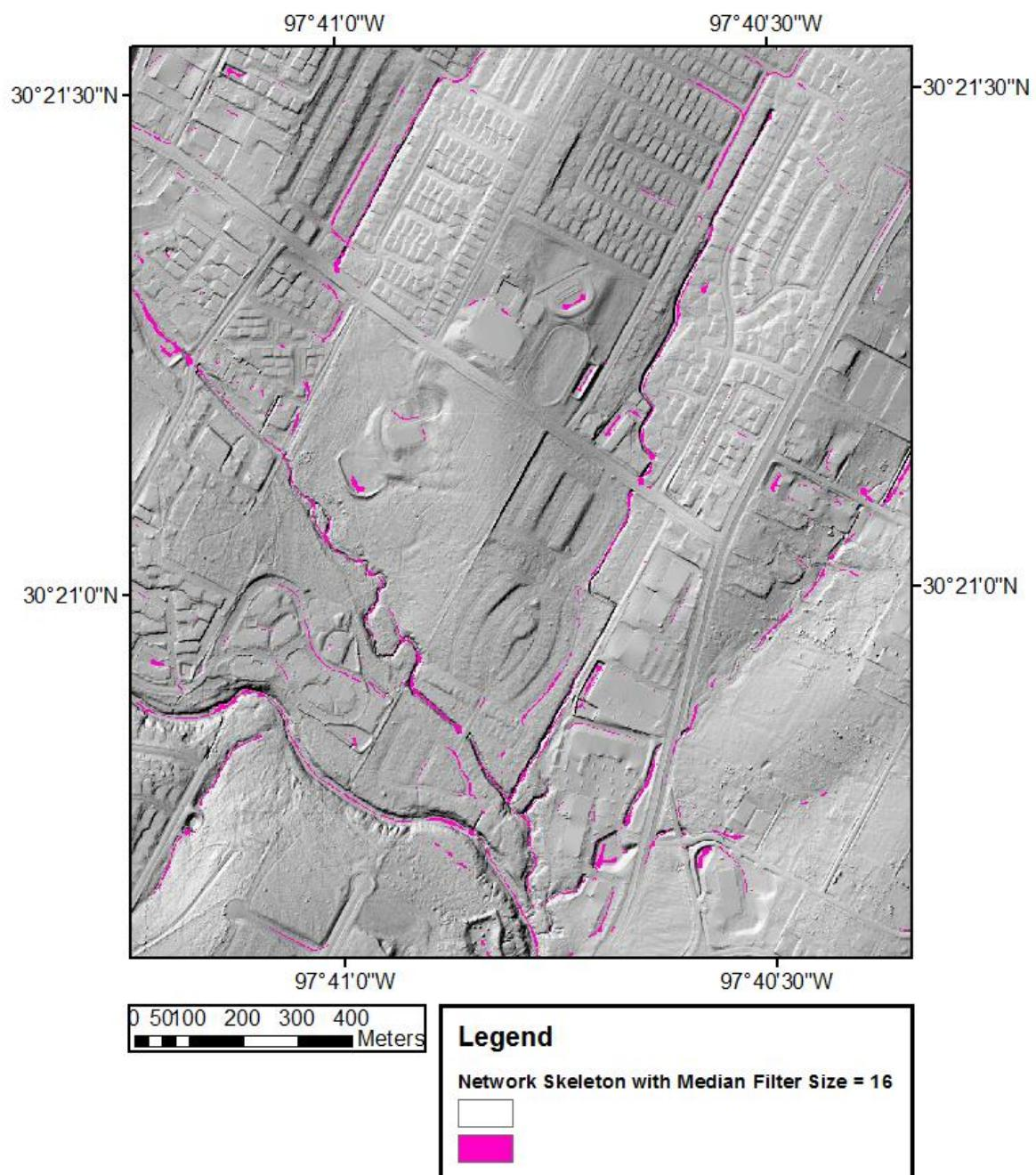
Figure 7. Channel skeleton results for median filter kernel size of 16 m (~1 road width).
