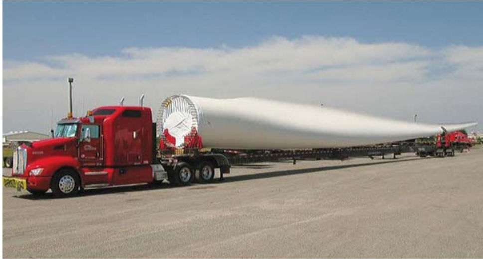
Figure 2.1: A truck hauls a massive 55-meter blade manufactured by Siemens Source: Del Franco (2014)
