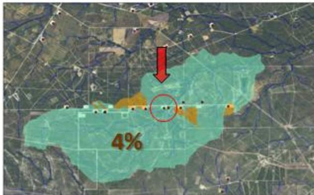
The red arrow points to a well pad that if sited differently or removed would reduce the potential for contamination by Hortonian flow over the drilling pad
