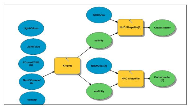
**Figure 2:** Geoprocessing model built using model builder to perform interpolations of all measured parameters.
