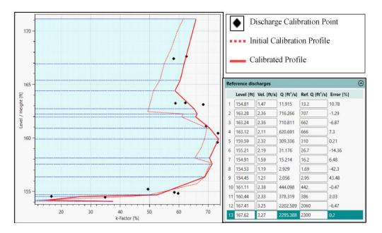
Figure 3.3.10 Example of a 13-point calibration of the k-factor profile in Q-Commander
