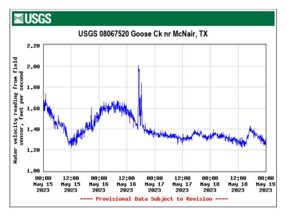
Figure 3.3.6 Example of the observed fluctuations in raw velocity
