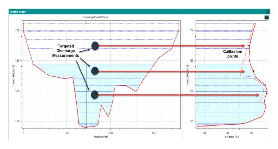
Figure 3.3.12 Channel geometries are targeted to constrain the k-factor profile
