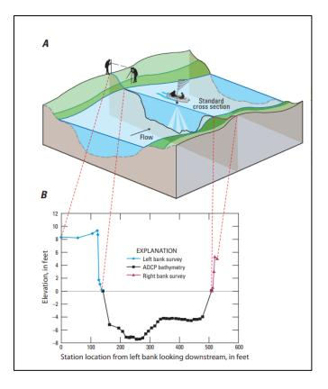
Figure 3.3.1 Example of a cross section survey involving multiple techniques (Levesque and Oberg, 2012)
