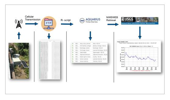
Figure 3.2.3 Transmission of data from the gauge to the public
