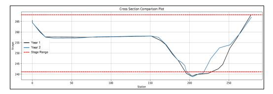
Figure 3.3.3. Example of a cross section comparison plot where channel modifications were made between surveys
