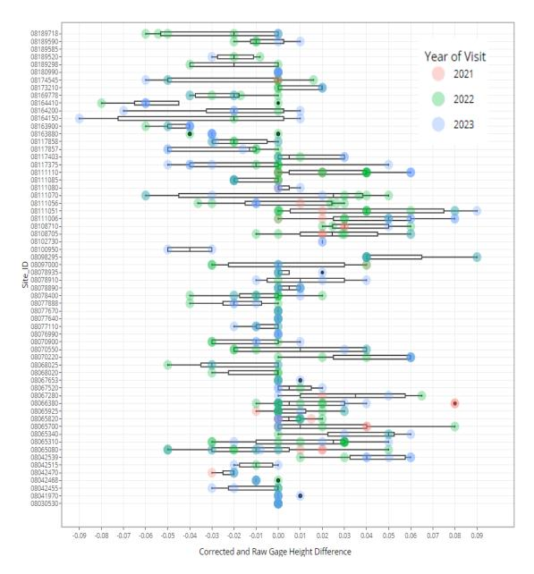
Figure 3.3.5 Box plot displaying the amount of drift observed at 53 stream gauges
