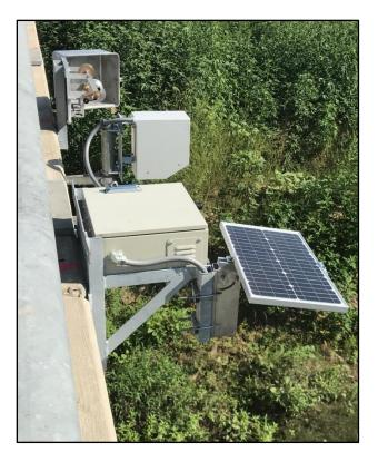
Figure 3.2.1. Image of a completed RQ-30 gauge installation
