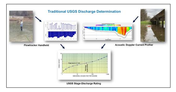
Figure 3.1.1 USGS Ratings are developed using direct field measurements to create a stage-discharge relation
