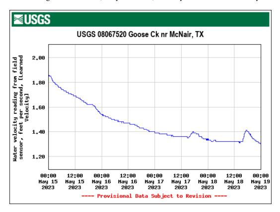
Figure 3.3.7 Example of how learned velocity can minimize velocity fluctuations
