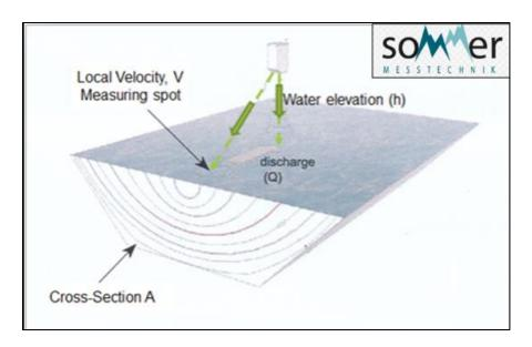
Figure 3.2.4 Conceptual drawing of an RQ-30 gauge sensor
