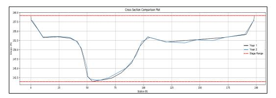
Figure 3.3.2. Example of a typical cross section comparison plot for computing differences in area
