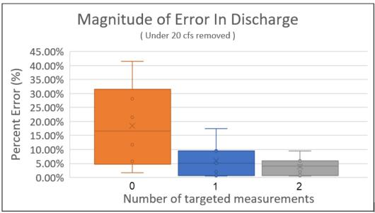
Figure 3.3.13 The magnitude of error for all measurements using the targeted calibration approach
