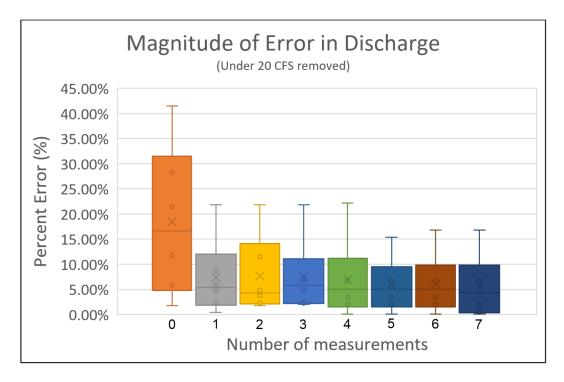
Figure 3.3.11 The magnitude of error between the RQ-30 computed discharge and the USGS verification measurements as calibrations are performed sequentially
